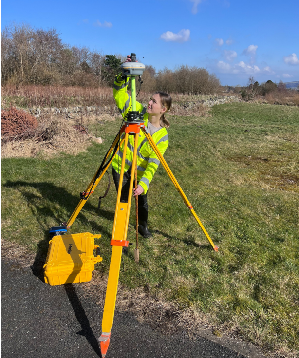
Here is Bethany setting up a base station for a topographical survey
